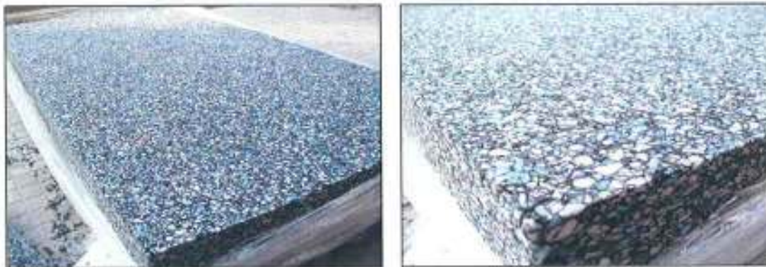
Images 1 and 2 – Details of the 40 mm Recfoam ® U80 panels
